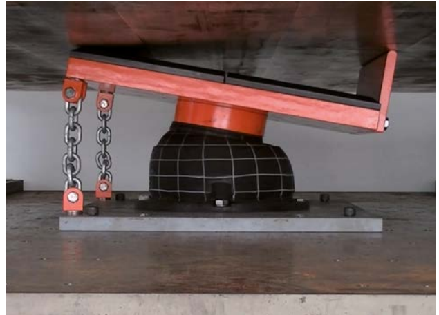
SPC Fender angular compression testing with restrain chains
