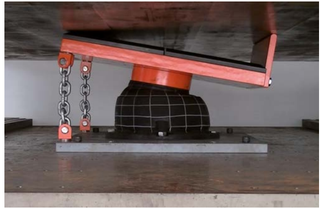
SPC Fender angular compression testing with restrain chains
