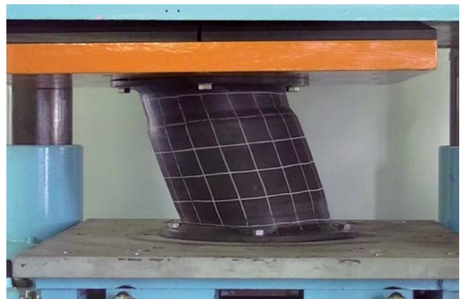
CSS Fender shear testing with panel and UHMW-PE face pads
